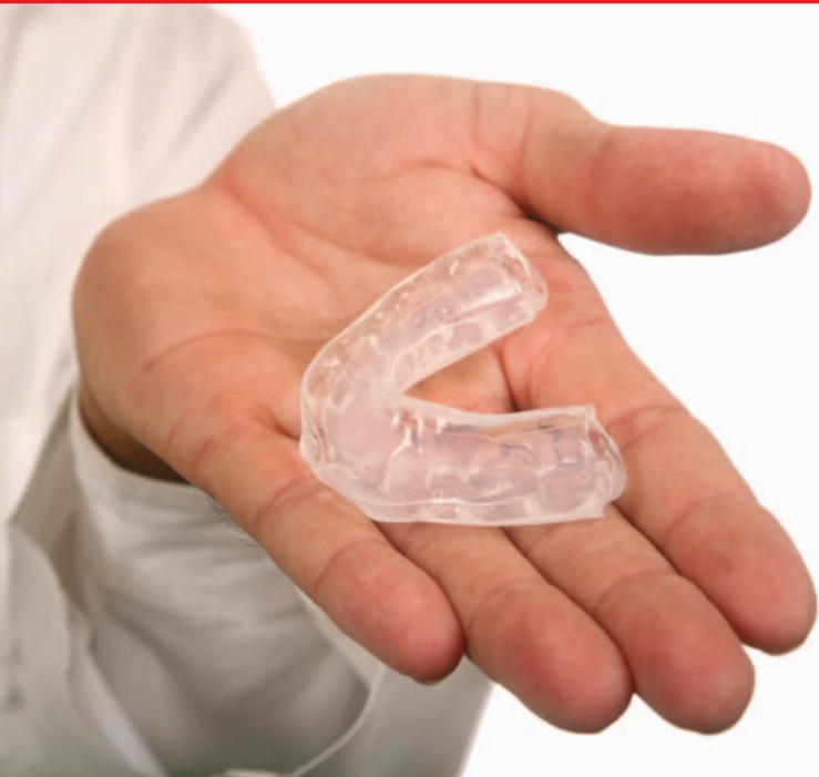
Picture 3: Mouthpiece insert as a finished part example after the thermoforming process
