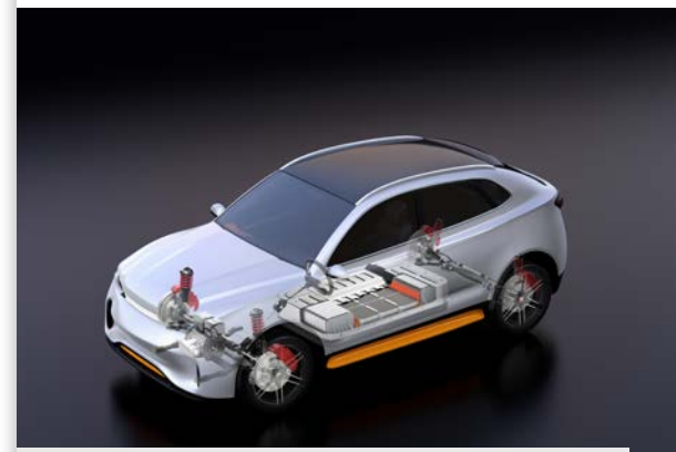
Lithium battery pack in an electric car (image: stock.adobe.com)
