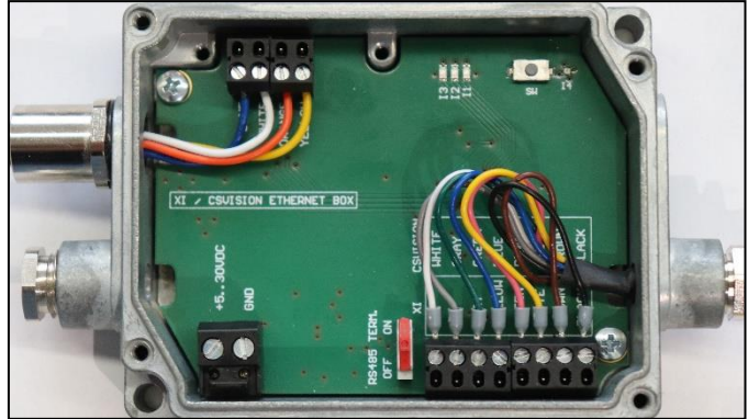
Installation of the Network Interface board
