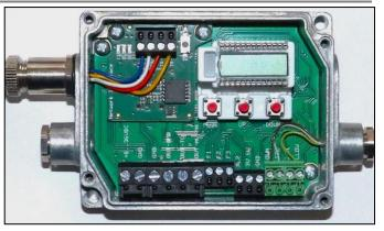
Installation of the Network Interface board into Optris CT Electronic Box
