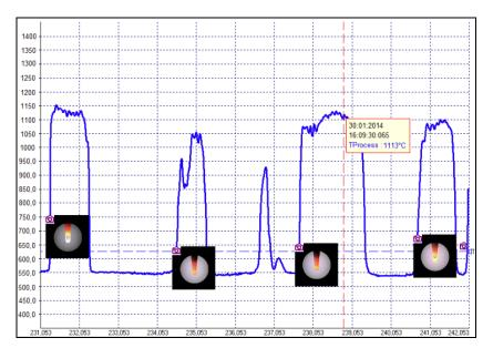
Temperature-Time-Diagram with automatic snapshots – a mouse click on the camera icon opens a thumbnail of the according picture; double click opens the snapshot in full screen.
