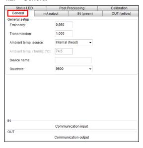
**Emissivity** Emissivity setting (Fixed value)
