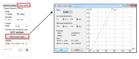
Alternatively the output channel 1 can also be used as an alarm output. Thereto you have to choose the mode **digital**. The selection **Normally open/ closed** defines the output as High or Low alarm.
