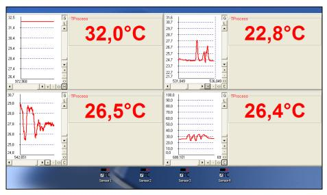
Four displays with diagrams are showing the temperature of four via USB connected sensors
