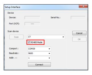
For a faster data transfer we recommend the **RS422 mode**. You will need also the RS485 module and the RS485-USB adapter [ACCTRS485USBK]. To activate the RS422 mode you have to call this function with the programming keys on the sensor at first (menu item: multidrop address). Now you can connect the sensor as described under ▶ **Connection Sensor – Computer**. The RS485 Mode must be deactivated in this case.
