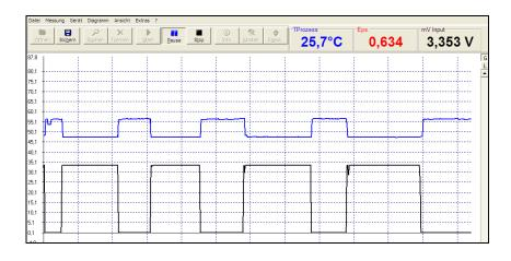
Example: External emissivity setting via an analog voltage at the pin IN/ OUT. The graph allows an analysis of the process temperature change in dependence on the set emissivity.
