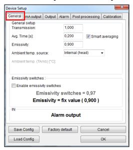
Transmission: Transmissivity setting
