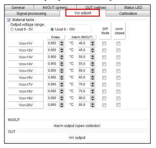
If this function is activated you can switch between 10 different emissivity settings combined with alarm threshold values by variation of the supply voltage (Vcc).
