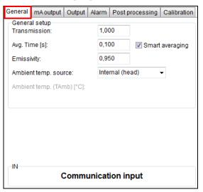
Transmission: Transmissivity setting
