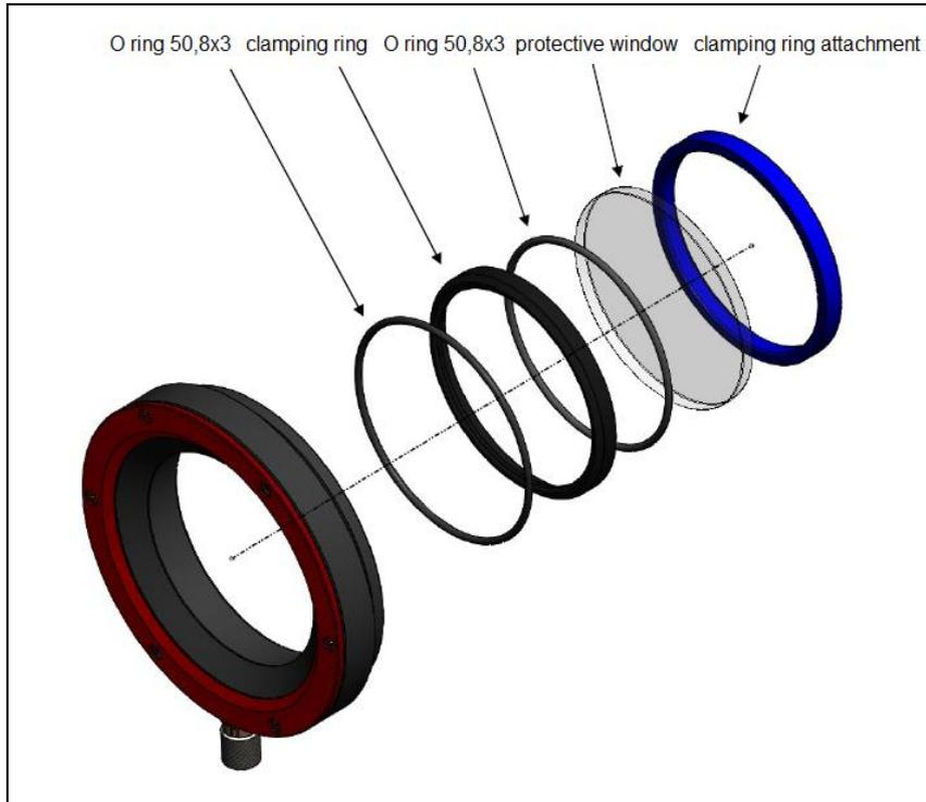
Figure 31: Assembly protective window
