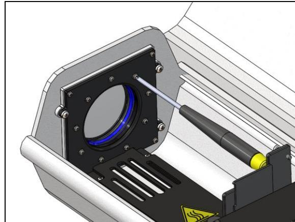
Figure 23: Loosen 9 screws from the adapter plate
