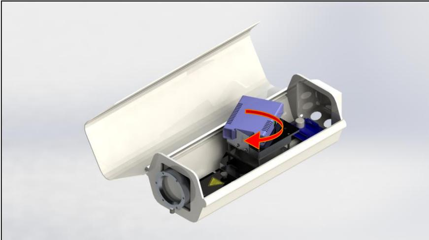
**Figure 6:** Insertion of the USB server into the provided board
