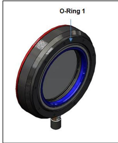
**Figure 30:** Insert O-ring 1 in air purge collar
