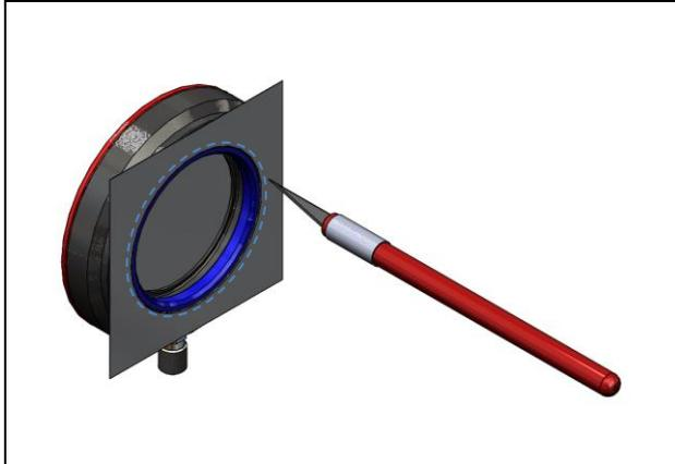
**Figure 27:** Cut the protective foil with the scalpel
