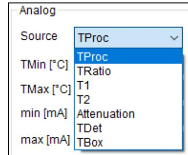
The desired temperature measuring range of the sensor can now be set. The range limits can be changed by entering them in the corresponding fields. The source can be selected between **T<sub>Proc</sub>**, **T<sub>Ratio</sub>**, **T<sub>1</sub>**, **T<sub>2</sub>**, **Attenuation**, **T<sub>Det</sub>** or **T<sub>Box</sub>**.
