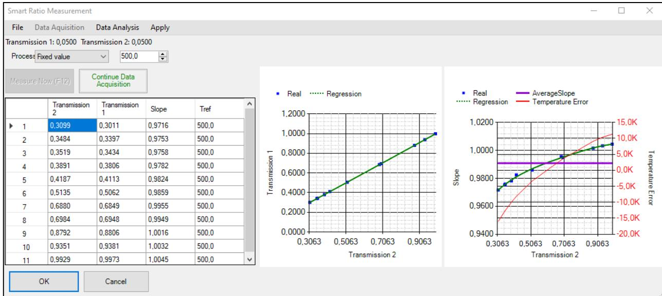
Smart ratio mode is now activated. Further data points can no longer be recorded in this mode. To add more data points, press the **Continue Data Acquisition** button (Smart Ratio mode is deactivated again).
