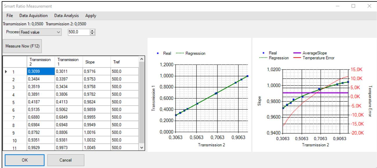
Smart Ratio example with 11 measuring points
