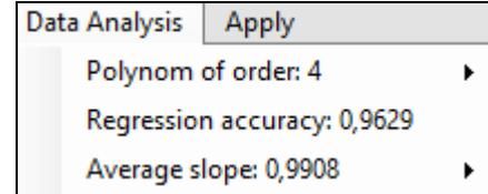
**Regression accuracy:** Characteristic value to evaluate the description of the measured values by the polynomial. Larger values are better. A value of 1 means perfect agreement. The regression accuracy is calculated automatically.
