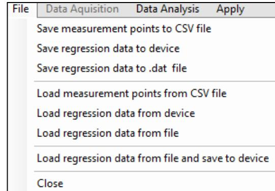
**Save regression data to .dat file:** Here the data is stored on a hard disk for external data analysis.
