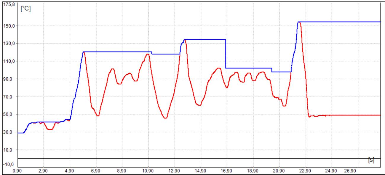
—  $T_{Proc}$  with Advanced peak hold (Threshold = 80 °C/ Hysteresis = 20 °C)
