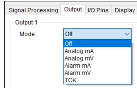
When using the analog mA or mV output, either  $T_{Proc}$ ,  $T_{Int}$  or  $T_{Box}$  can be selected as source. The desired temperature measurement range of the sensor can now be set. The range limits can be changed by entering the values in the corresponding fields.
