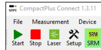
Activation of the Smart Ratio function is indicated by a green illuminated **On** button. In addition, there is an icon called **SRM**, which is framed in green when activated.
