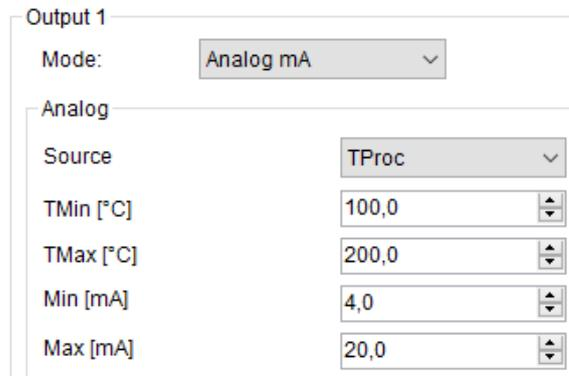
Alternatively, outputs 1 and 2 can be used as alarm outputs. To do this, select the **Alarm mA** or **Alarm mV** setting.
