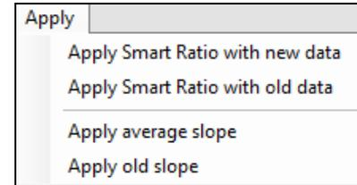
**Apply Smart Ratio with old data:** Regression curve already stored in the device is retained and Smart Ratio mode is activated.
