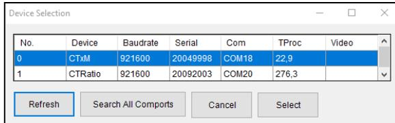
**Example 2:** Two sensors were found. Please activate with the cursor the desired unit and after that press the **Select** button to close the window.
