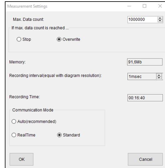
**Recording time** Maximum time of measurement, calculated from **Max data count** and **Recording interval**
