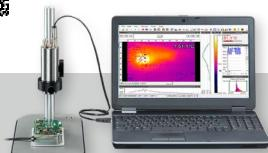
Infrared camera of the Compact Line Xi 400 microscope optics
