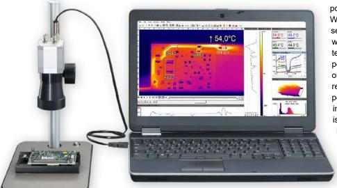
Temperature measurement of smallest components www.optris.com ELECTRONICS INDUSTRY
