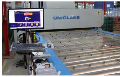
Temperature monitoring of glass sheets in a tempering machine
