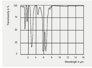
Spectral transmissivity of air (1 m, 32 °C (90 °F), 75 % r. F.)
