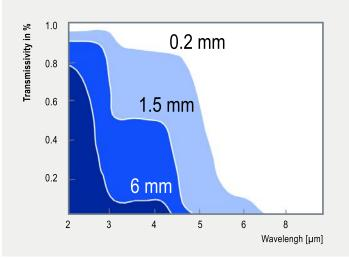
Spectral transmissivity of glass depending on the thickness
