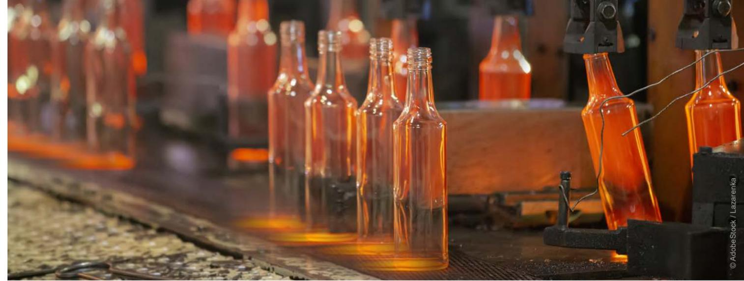
During the **forming process**, which takes place at temperatures of over 500 °C (932°F), infrared sensors are also used for monitoring. Since the process only takes a few seconds, the reaction of the sensors is of critical importance here. The thermal measurement of the glass can be influenced by direct measurement of the glass surface or indirect measurement of the surface of the forming tool for both the forming of the parison shape as well as during finishing of the mold.
