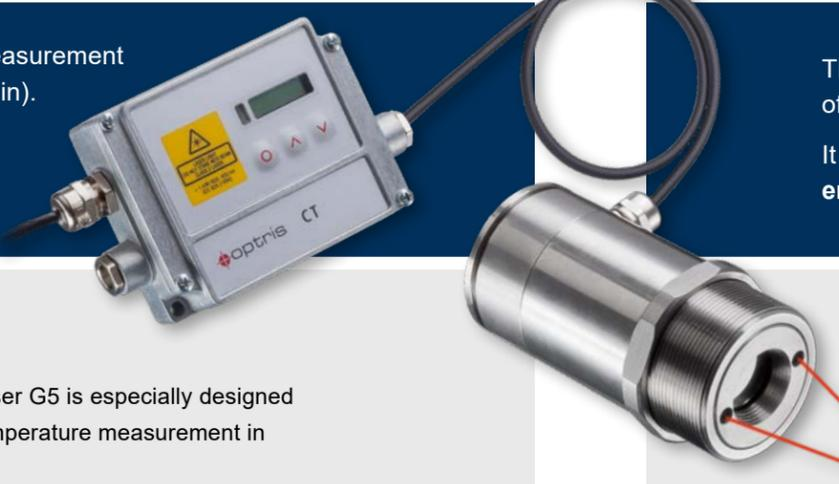
The infrared thermometer optris CTlaser G5 allows the temperature measurement of **smallest objects of 1 mm (0.04 in)** from a distance of 70 mm (2.76 in). Due to its **very short response time** of 10 ms it is often used for fast processes.
