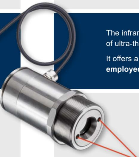
The infrared thermometer optris CTlaser G7 is perfectly suited for precise temperature measurement of ultra-thin glass surfaces. It offers a broad temperature range from 100 °C up to 1200 °C (212 °F to 2192 °F) and **can be employed in temperatures of up to 85°C (185 °F) without additional cooling**.
