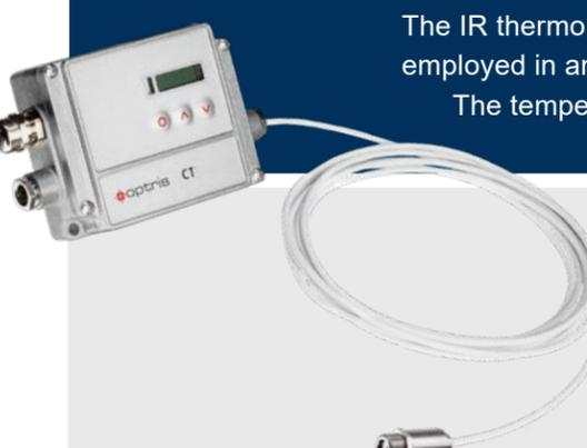
The IR thermometer's stainless steel measuring head is **extremely small** and can be employed in ambient temperatures of up to 85 °C (185 °F) without additional cooling. The temperature range is from 100 °C to 1650 °C (212 °F to 3002 °F).
