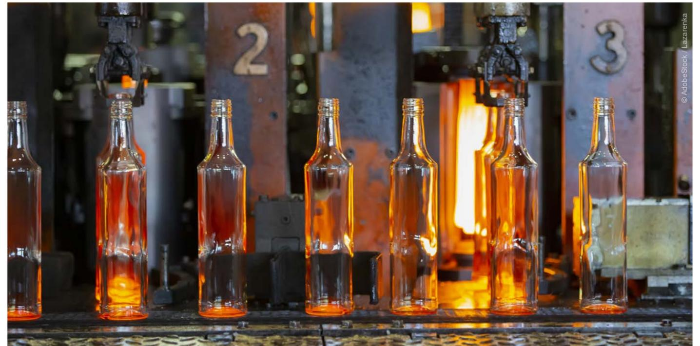
Temperature measurement for quality control after the forming process
