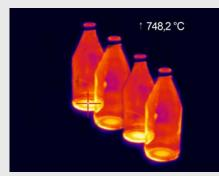
Hot-spot measurement in the production of glass bottles
