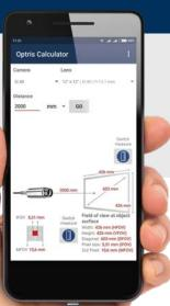
The measuring spot size of the respective device is calculated for each distance
