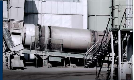
Application example: rotary kiln in the chemical industry
