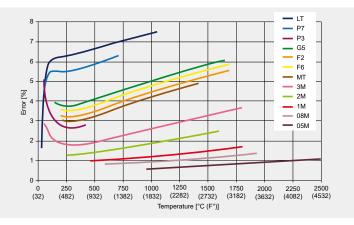
Measuring error in the case of emissivity wrongly adjusted by 10% as a function of the wavelength and object temperature (LT:  $8-14 \mu m$ ; P7: 7.9  $\mu m$ ; P3: 3.43  $\mu m$ ; G5: 5 µm; MT: 3.9 µm; F2: 4.24 µm; F6: 4.64 µm; 3M: 2.3 µm; 2M: 1.6 µm; 1M: 1.0 µm; 08M: 800 nm; 05M: 525 nm)
