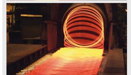
Hot working of sheet metals and manufacturing of wire
