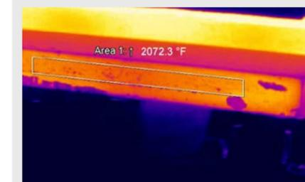
Run-off area of a continuous casting plant
