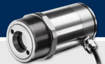
The optris CTlaser 05M / 1M / 2M / 3M infrared thermometers were **specifically developed for the temperature measurement of metal surfaces and molten metals**. They feature short-wave spectral ranges of 525 nm (05M), 1 µm (1M), 1.6 µm (2M) and 2.3 µm (3M), which also minimize measurement errors in the case of changes in emissivity. The temperature ranges of the thermometers are between 50 °C and 2200 °C.
