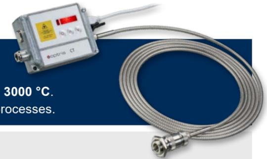
With the **ratio pyrometers** of the **CSvision** family, it is possible to measure temperatures of metals non-contact, safely and reliably in a range **from 250 °C up to 3000 °C** from variable distances. The **novelty of the CSvision series** is the **switchable two-step brightness reduction filter**, which makes it easy to sight and focus on very bright objects.
