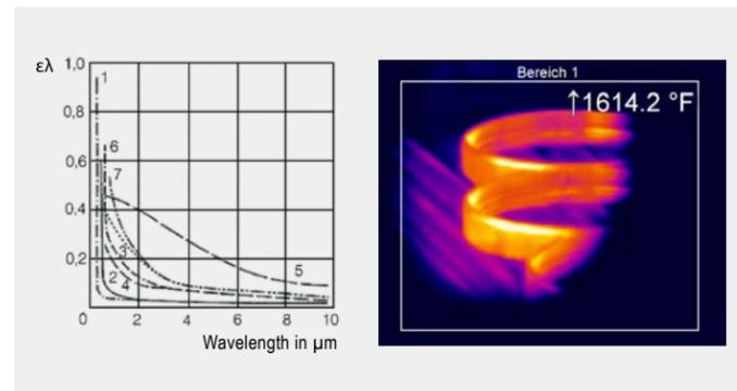
Measuring of bearing rings during the hardening process
