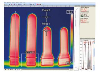
In-depth inspection of preforms during bottle production.
