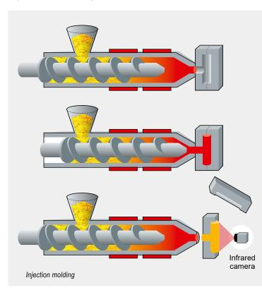
Injection molding is the most common production process in the manufacture of moldings from thermoplastic polymers. It is used in particular in the intermittent mass production of complex moldings where the size of the workpieces ranges from the smallest of cogs right up to large containers. The weight of a workpiece starts at 1 mg (0.001 g) and goes up to 100 kg.
