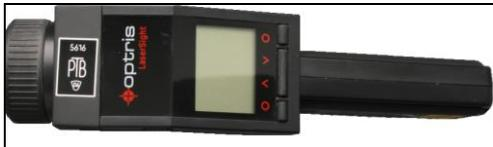
Transfer standard IR thermometer LS-PTB
