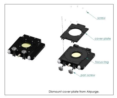
Figure 51: Assembly of the laminar air purge
