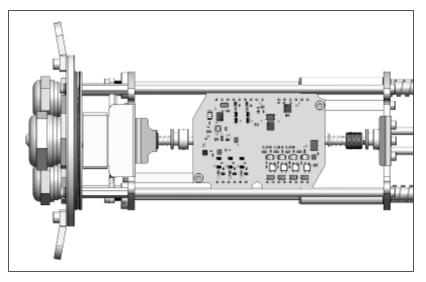
Figure 38: Mounting of the industrial PIF (top view)
