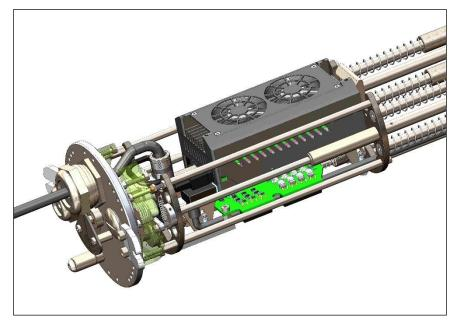
Figure 43: Mounting USB and network connector to NetBox
