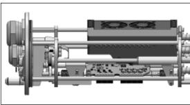
Figure 41: Fitting the PI NetBox into the chassis (right hand view)
