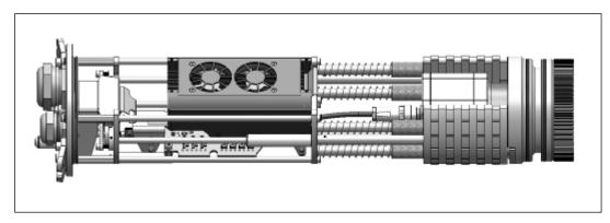
Figure 42: Chassis with PI camera, industrial PIF and PI NetBox
