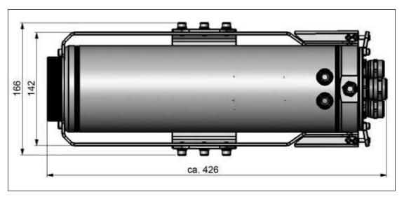
Figure 11: CoolingJacket Advanced, extended version – top view
