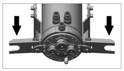
Figure 32: Unlocking of the hinge
