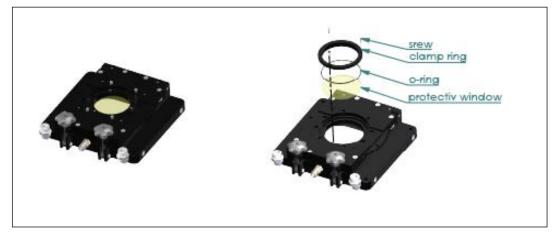
Figure 54: Change of the protective window
