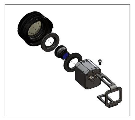
**Note:** For the installation of the 80 ° and 90 °optics, the camera must be fixed upside down on a supplied bracket.
