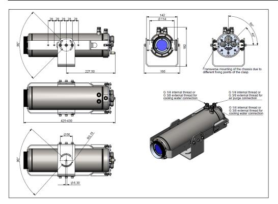
Figure 13: CoolingJacket Advanced, extended version - complete view
