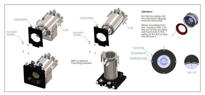
Figure 52: Assembly of the laminar air purge
