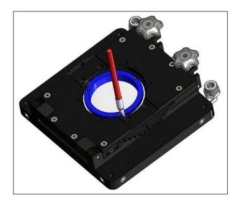
**Step 6:** Now place the O-ring in the groove of the blue ring.
