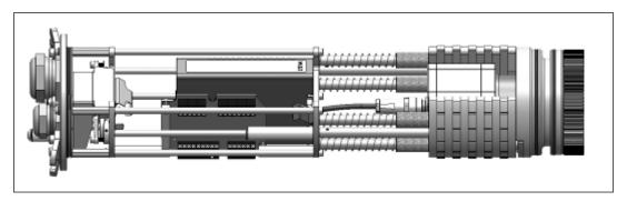
Figure 47: Chassis with PI camera, industrial PIF and USB server Gigabit
