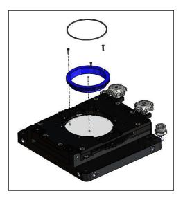
**Step 3:** Place the blue ring centrally on the foil. Make sure that the holes for the screws are on top of each other.
