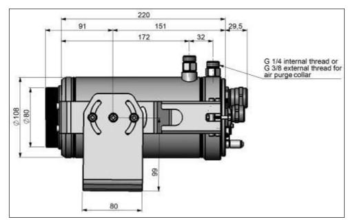
Figure 6: CoolingJacket Advanced, standard version - side view
