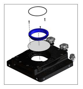
**Step 2:** Place the foil centrally in the circular shoulder of the upper plate.
