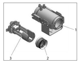
Figure 24: CoolingJacket Advanced, standard version
