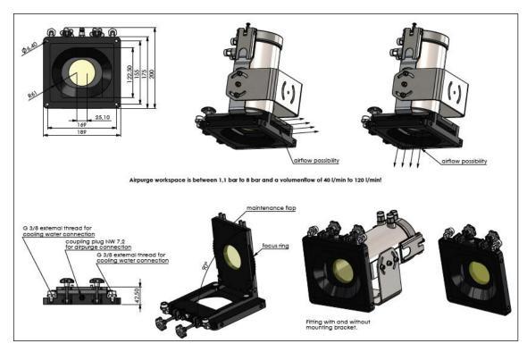
Figure 3: Dimensions of laminar air purge
