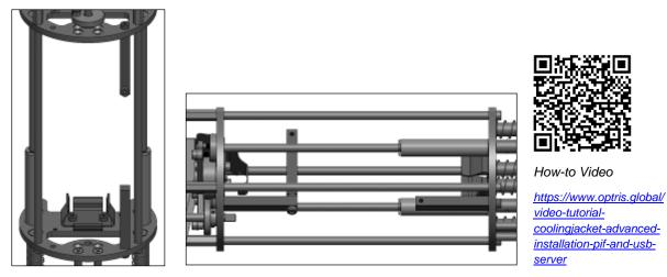
**Figure 44 (a + b):** Mounting of the accessories for USB server Gigabit: **a)** DIN rail plate for USB server Gigabit (view from the bottom), **b)** Support rods for industrial PIF (right hand view)
