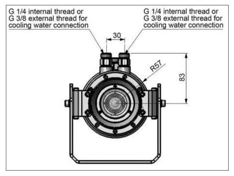
Figure 12: CoolingJacket Advanced, extended version - front view
