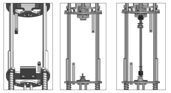
**Figure 37 (a-c):** Mounting of the accessories for PI NetBox: **a)** Holding plate for PI NetBox (top view), **b)** Support rods for industrial PIF (view from the bottom), **c)** Shaft to fix the PI NetBox (view from the bottom)
