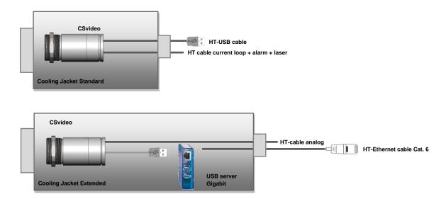
\*All high temperature cables are available for temperatures up to 180 °C/ 250 °C:
