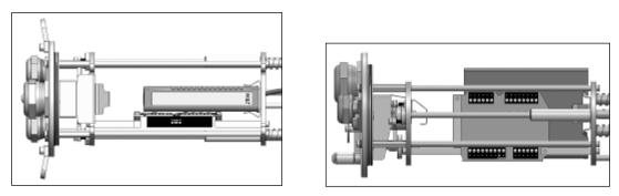
Figure 46 (a + b): Fitting the USB server Gigabit into the chassis (top view and right hand view)
