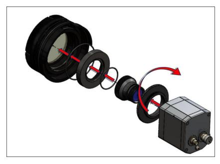
Figure 18: Assembling of the focusing unit
