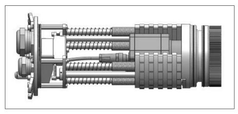
Figure 28: Focusing unit with camera
