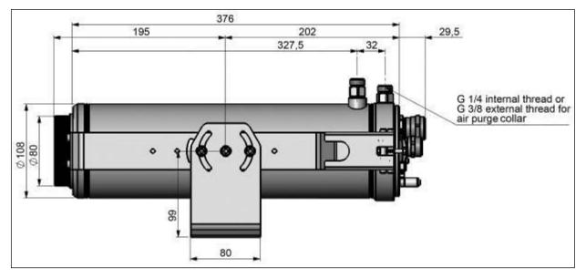
Figure 10: CoolingJacket Advanced, extended version – side view
