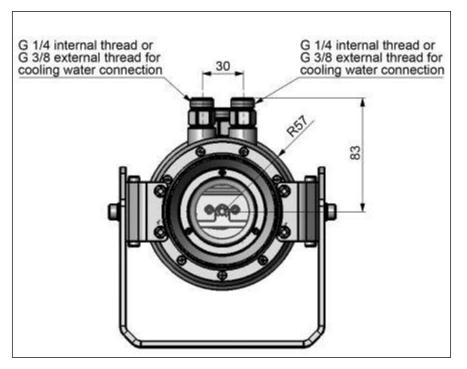
Figure 8: CoolingJacket Advanced, standard version - front view
