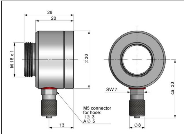
**Air purge collar for massive housing (thread M18x1)
