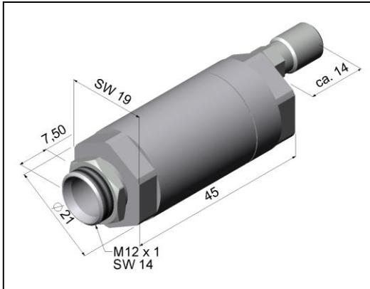
**Standard air purge collar [ACCTAP] for optics with a D:S  $\geq$  10:1 (not for sensing heads with 32 mm length), fits to the mounting bracket
