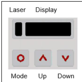
Pressing the Mode button again recalls the last called function on the display. The signal processing features **Peak hold** and **Valley hold** cannot be selected simultaneously.
