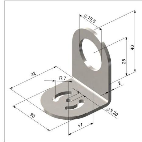
**Mounting bracket for massive housing,
