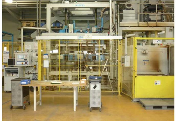
A Kiefel deep-drawing system is used for the production of panel parts at the Gubesch Group.
