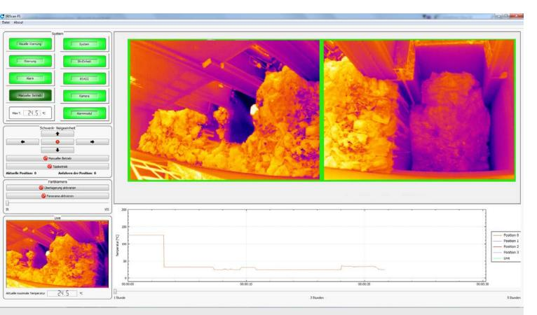
Using the flexible IRISvisual software, the parameters, for example such as the temperature thresholds, can be adjusted very simply. If the multi-stage temperature thresholds are exceeded, the system automatically triggers the corresponding alarm.
