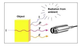
Figure 50: Composition of IR radiation
