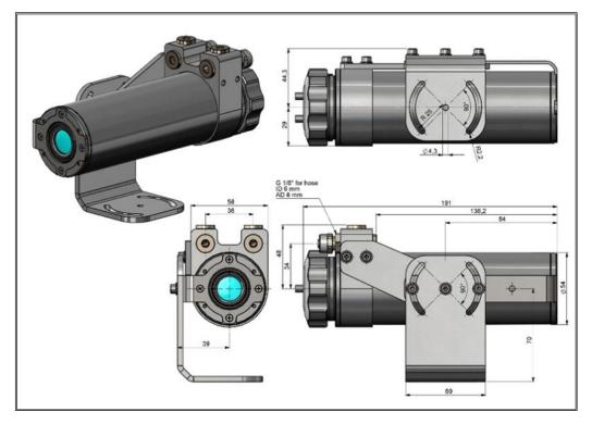
Figure 14: Water cooling (ACXIMW) and mounting kit (ACXIxxxWAK1), dimensions [mm], weight: 1710 g
