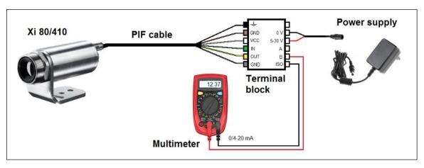
Figure 40: Electrical installation for autonomous operation Xi 80/410/410 MT/1M
