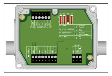
Figure 18: Control box of shutter, dimensions (see Figure 9)
