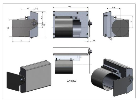
Figure 15: Shutter for water cooling (ACXISW), dimensions [mm], weight: 600 g
