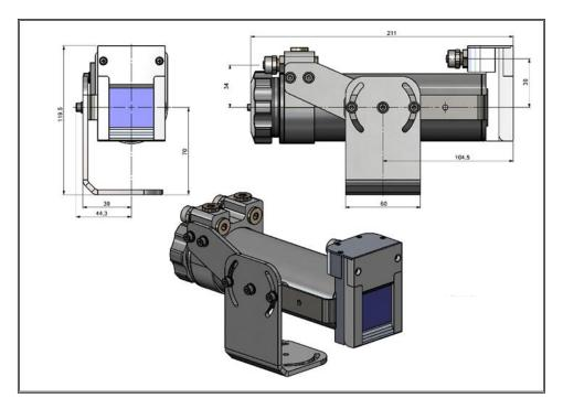
**Figure 19:** Air purge (ACXIAPL), water cooling (ACXIMW) and appropriate mounting kit (ACXIxxxWAKx), dimensions [mm]
