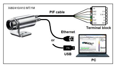
Figure 36: Connection Xi 80/410/410 MT/1M to PC via Ethernet/USB
