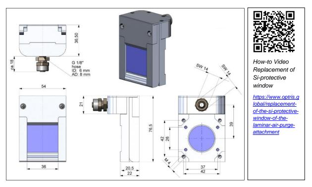
Figure 10: Laminar air purge with Si-protective window [ACXIAPL and ACXIMTAPL], dimensions [mm]
