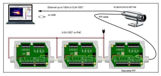
Figure 31: Connection of 3 industrial PIFs via RS485
