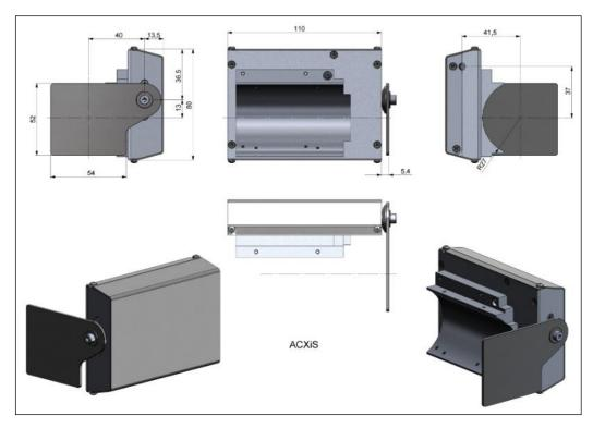
Figure 17: Shutter (ACXIS), dimensions [mm], weight: 550 g
