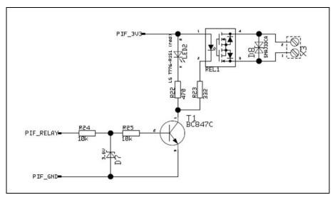
Figure 58: Relay output at industrial PIF
