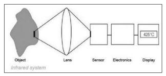
Figure 48: Main principle of non-contact thermometry
