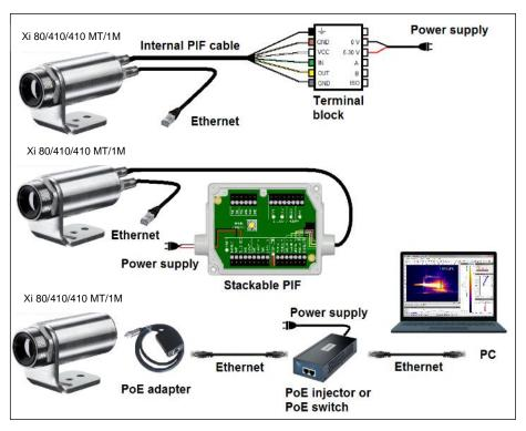
Figure 35: Possibilities of power supply for Xi 80/410/410 MT/1M via Ethernet connection
