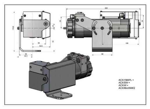
**Figure 20:** Air Purge (ACXIAPL), water Cooling (ACXIMW), Shutter (ACXISW) and appropriate mounting kit (ACXIxxxWAKx), dimensions [mm]
