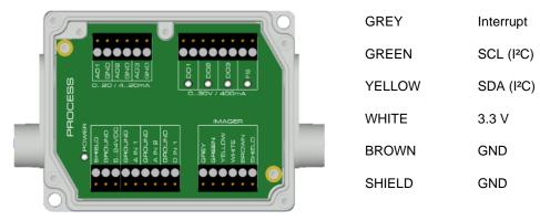
Figure 32: Connections of the industrial Process Interface for Xi 400/640
