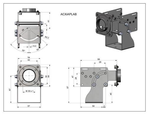
Figure 13: Mounting bracket (ACXIAPLAB), dimensions [mm], weight: 276 g
