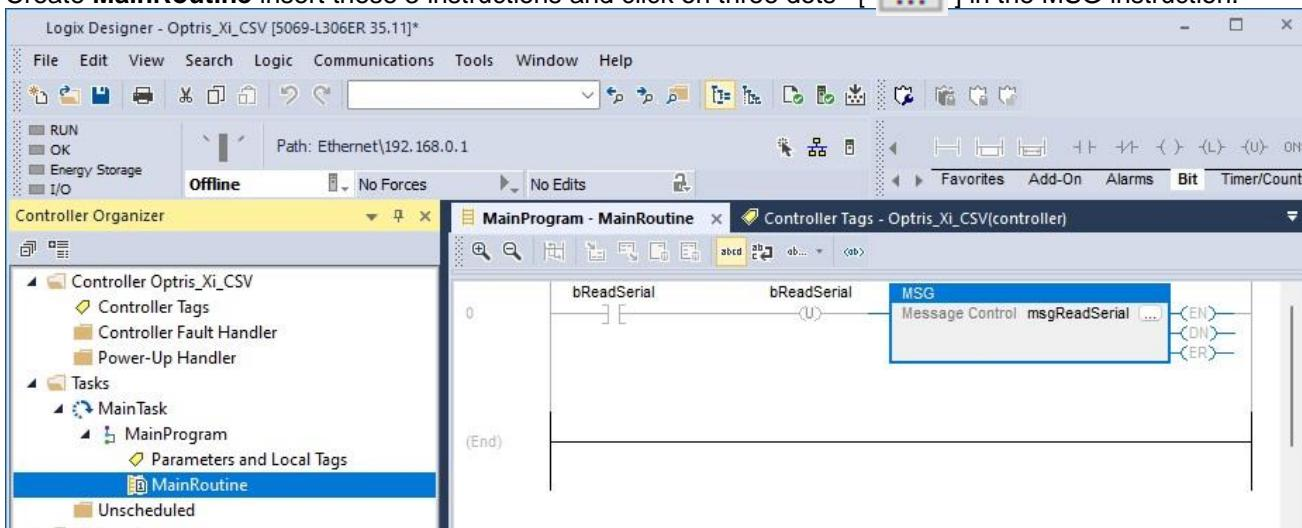
Set the configuration values according to **Table 3**, set the communication path to Opbris\_XI\_CSV, and click on **OK**. Download the project to the PLC and start the PLC program in **Run Mode**.
