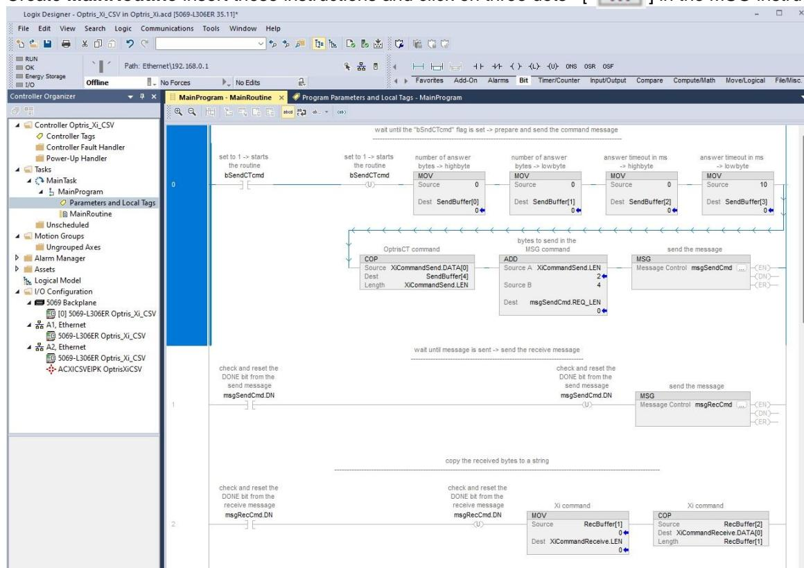
Set the configuration values like shown in the picture below, set the communication path to Optris\_XI\_CSV, and click on **OK**. Download the project to the PLC and start the PLC program in **Run Mode**.
