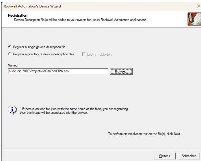
Click **next** until the message appears that the installation is completed and close the software "Rockwell Automation – Device Description File Installation Tool".
