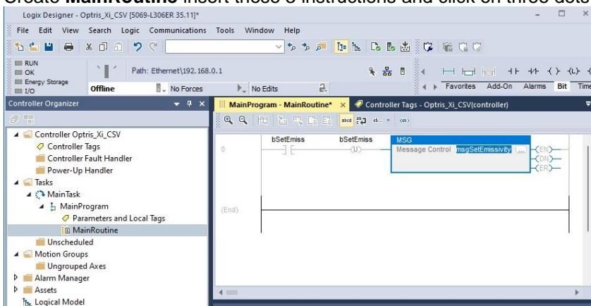
Set the configuration values according to **Table 3**, set the communication path to Opbris\_XI\_CSV, and click on **OK**. Download the project to the PLC and start the PLC program in **Run Mode**.
