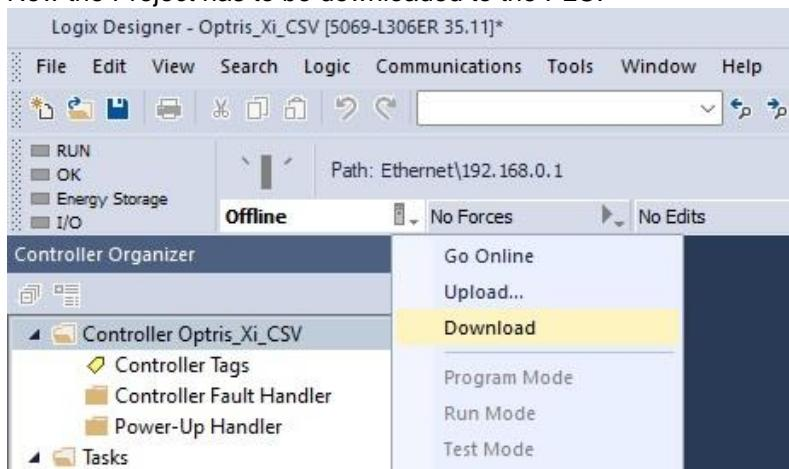
Start the PLC program by clicking **Run Mode**. To see the current cyclic values double-click on the **Controller Tags**.
