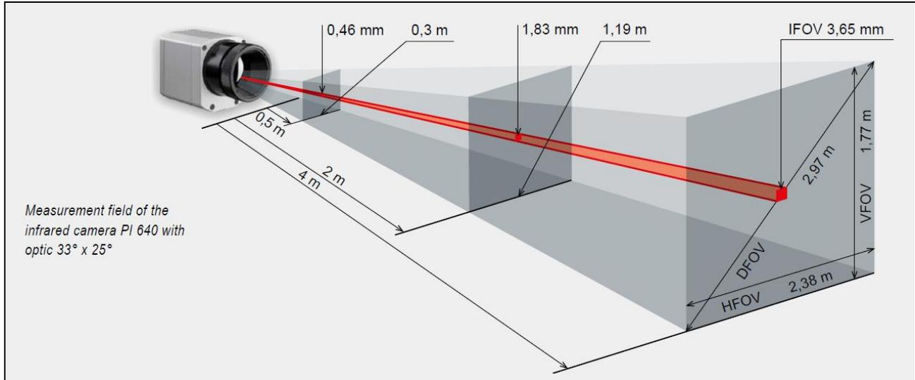
**Figure 4:** Measurement field of the infrared camera optris® PI 640 representing the 33° x 25° lens
