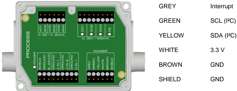
**Figure 28:** Connections of the industrial Process Interface
