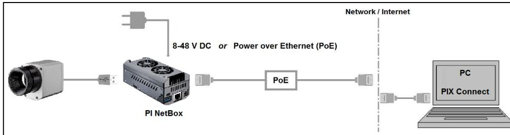
**Figure 32:** Ethernet network communication with PI Netbox
