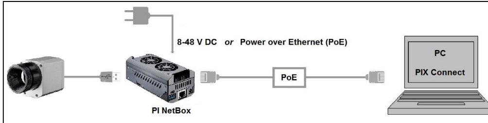
**Figure 31:** Ethernet direct communication with PI Netbox
