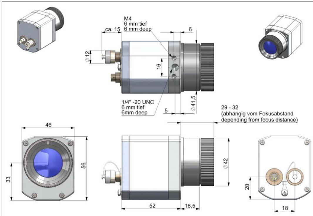
Figure 8: PI 640/ PI 640 G7, optics 80°/90°, dimensions [mm]
