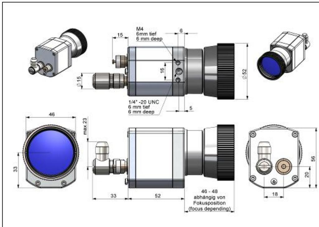
Figure 7: PI 640/ PI 640 G7, optics 13°/15°, dimensions [mm]
