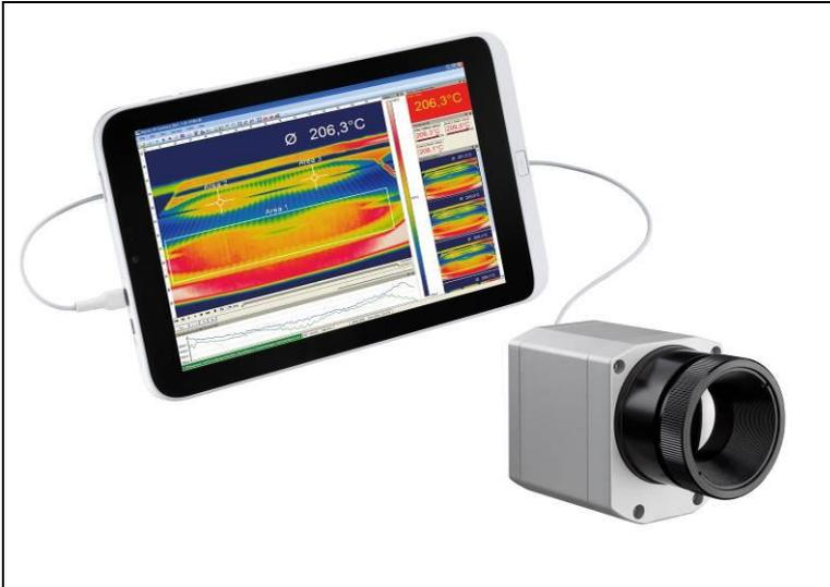
**Figure 40:** Non-contact thermometry
