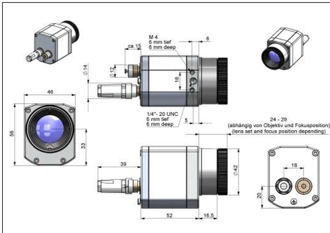
Figure 6: PI 640/ PI 640 G7, optics 29°/33° & 53°/60°, dimensions [mm]
