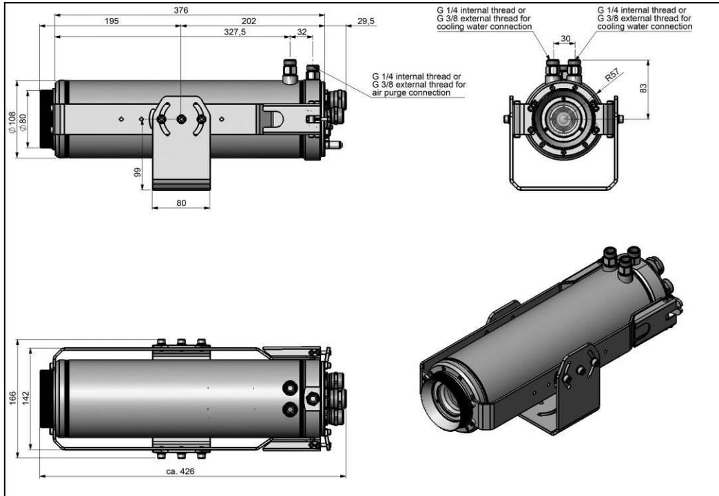
Figure 22: CoolingJacket Advanced [Part No.: ACPlxxxCJAE], Extended Version – Dimensions
