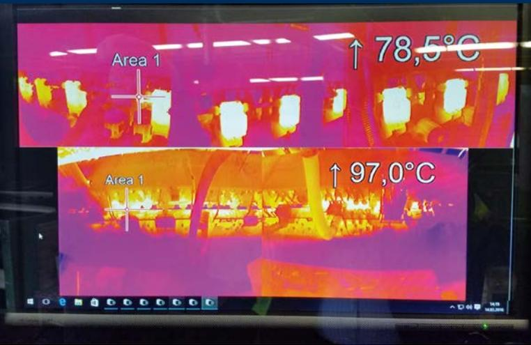
The PIX Connect software enables the overlapping of several heat images to form a total image / Merging Mode). The advantage is that the hottest point (Hotspot) can also be detected within the overall image
