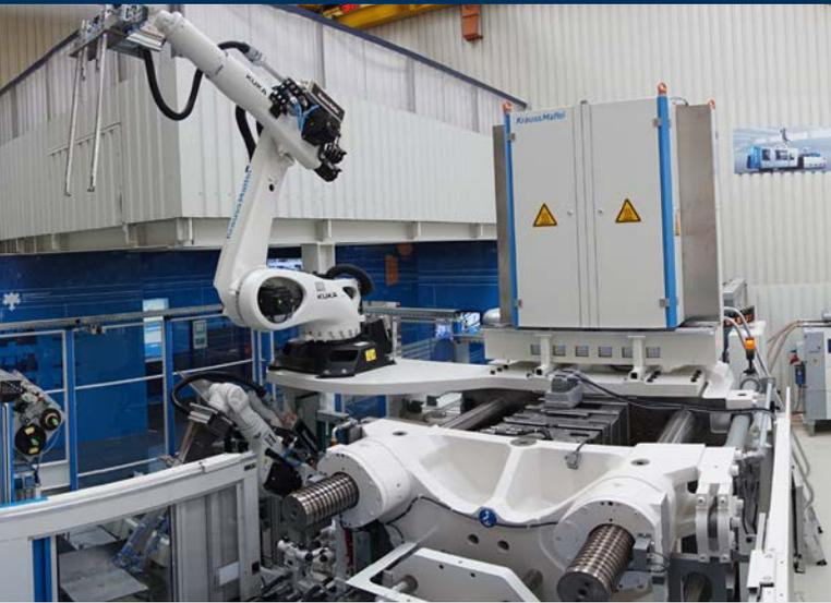
Automated manufacturing plan for the production of continuous fiber-reinforced thermoplastics.
